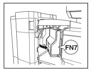
While holding open misfeed clearing guide FN8 (for finisher F-8430) or FN7 (for finisher F-8110), remove any paper.
